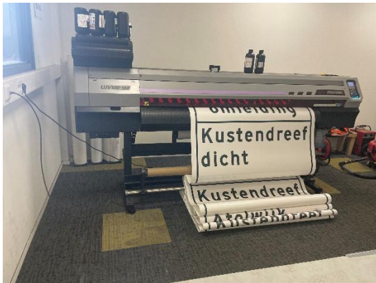
Figure 15 Foil printer used for printing on traffic signs
